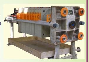
In the recessed type, the slurry is fed through the central inlet and the solids are retained in the recess between the plates, while the filtrate is collected through the corners.
